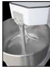
Tin coated cast iron knife and spiral. 304 stainless steel rotating bowl with anti-adherent treatment. Transmission system with chains and belts.
